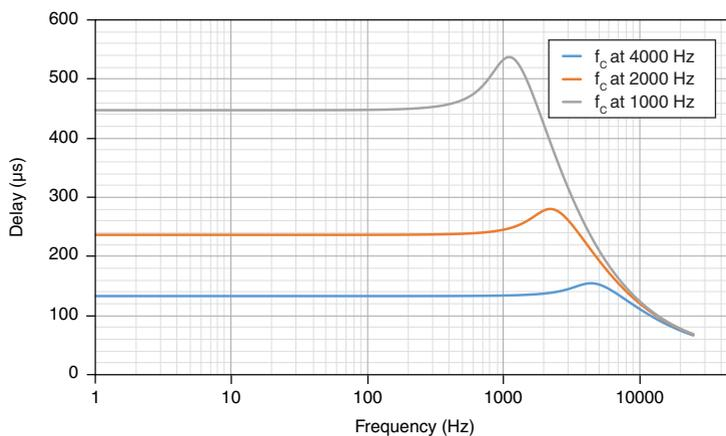
**Figure 6.** Butterworth Filter Input Delay (4th Order, with 12.8 MHz Timebase, 500 Hz, 250 Hz, 125 Hz)
