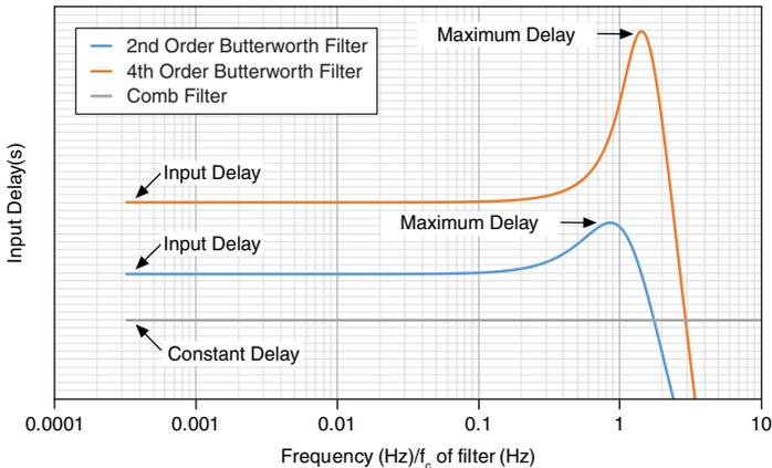
Each NI 9252 filter has a different frequency response to serve different applications:
